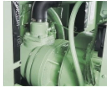
Rotary Screw Compressor Single-stage, fluid flooded. Cast iron housing is dimensionally stable, thick-walled and machined to close tolerances.
